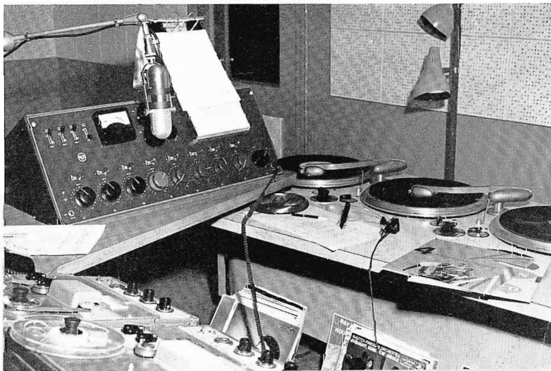
FIG. 8. Studio "A" (control room) is equipped with BC-3B console. Note two tape recorders on left, and three built in BQ-2B turntables at right.
