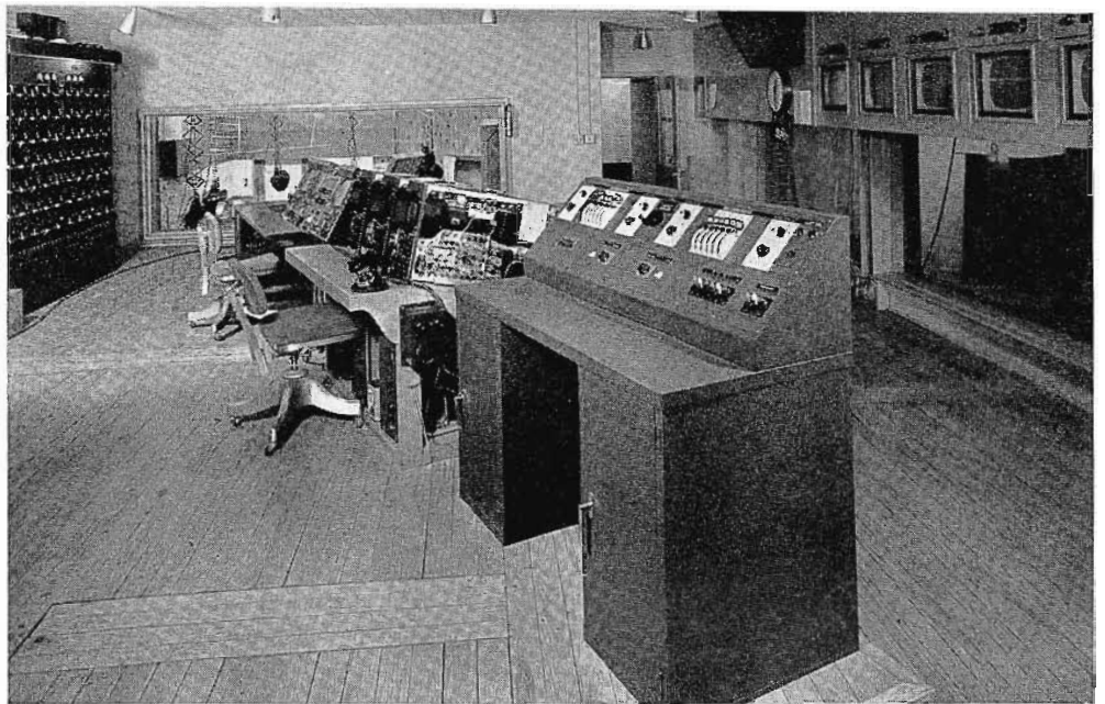
FIG. 12. The WTPA control room includes portable control units for three field cameras and controls, and two film cameras. Also housed here are lighting controls for both studios.
